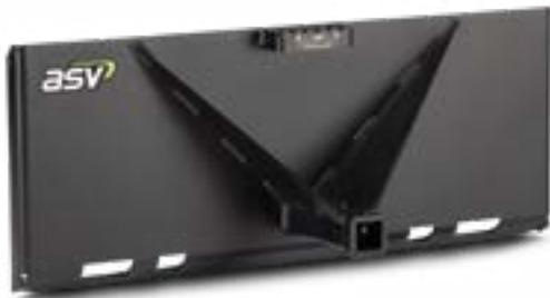
A receiver hitch plate allows you to conveniently maneuver equipment, especially in tight spaces, without additional manpower.
