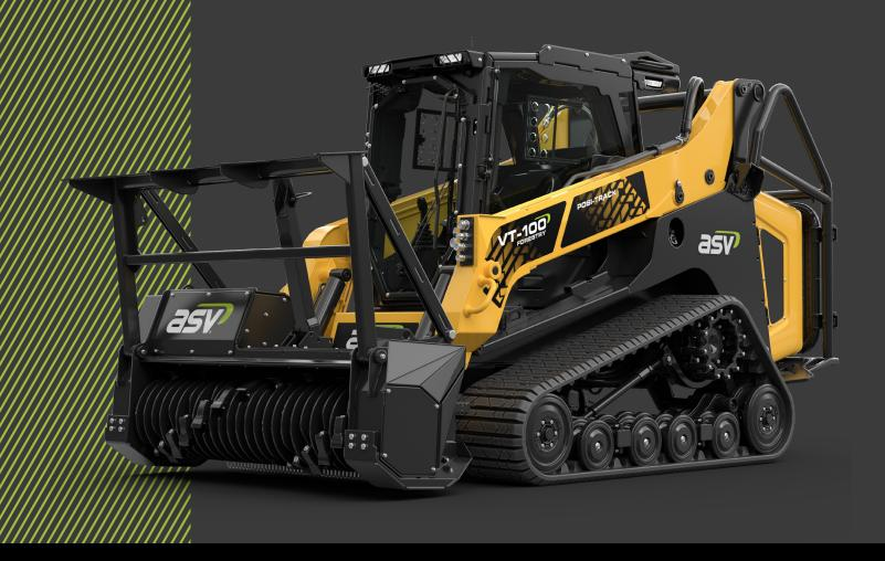
The Yanmar-powered MAX-Series™ VT-100 Forestry Posi-Track® loader is your answer to forestry-grade performance in a 103.5 hp compact track loader. From guarding that meets forestry safety standards to hydraulic flow and cooling capacity to keep up with demanding attachments, you'll take on land-clearing jobs with ease.
