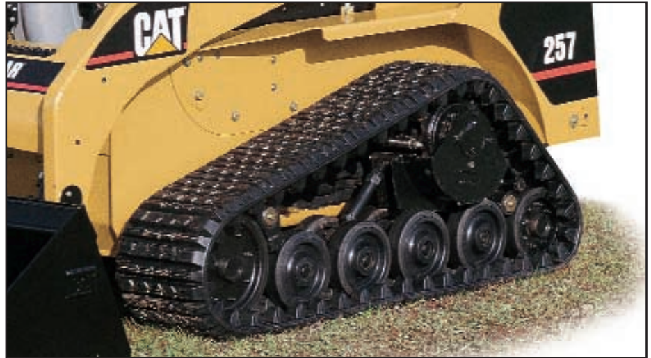
RT•50 Undercarriage on on Caterpillar 257 Multi Terrain Loader
